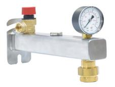
Safety group DHW is an important element of the hot water installation, whose main task is to protect the installation against the increase in pressure caused by the increase in water temperature in the system. It is intended for installation in home heating systems. The beam is equipped with a 6 bar safety valve, a pressure gauge and a set of mounting pins. Additionally, in the lower part of the beam there are connections for the expansion vessel and the power supply from the safety beam.
