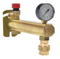
DHW safety group is an important element of the hot water installation, whose main task is to protect the installation against the increase in pressure caused by the increase in water temperature in the system. It is intended for installation in home heating systems. The beam is equipped with a 6 bar safety valve, a pressure gauge and a set of mounting pins. Additionally, in the lower part of the beam there are connections for the expansion vessel and the safety beam supply.
