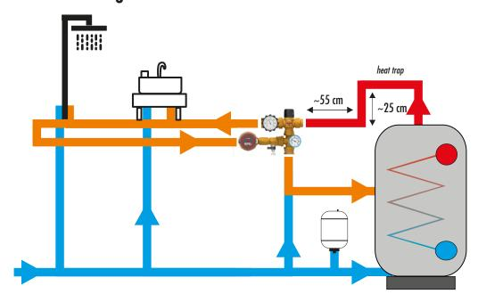
Simplified schematic diagram of the installation - the standard ones were not marked installation elements as well as the boiler room security scheme.
