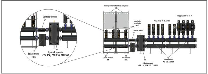
In order to facilitate the periodic cleaning of the installation, it is recommended to mount the shut -off valves before and for basket strainer.
