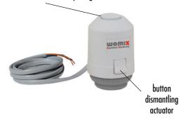
The MP VM200 thermoelectric actuator is a drive for opening and closing valves on underfloor heating manifolds. The set includes an adapter that allows the device to be mounted on thermostatic valves in CS-Rot manifolds. The adapter allows for quick installation of the actuator only by pressing it and subsequent disassembly of the actuator only by using the disassembly button. The actuator is in the normally closed position, after applying voltage it opens the valve flow.
