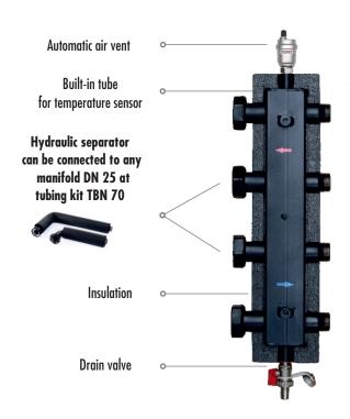
The CPN 70 2F - DN 25 hydraulic separator is made of steel. The factory is equipped in insulation, from the top in the connection for the vent (1/2 "socket) and a built-in pipe for the temperature sensor and from the bottom in the drain connection (1/2 "socket). The set includes a 3/8 "vent with a 1/2 "foot valve, a 1/2 "drain valve, four 1 "cast iron fittings and wall brackets.
