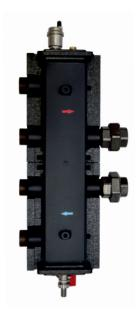
Hydraulic separator **CPN 100 2F - DN 32** is made of steel. The factory is equipped with insulation, on the upper side with two connections for a temperature sensor and a vent and on the lower side with a drain connection. Included There are a air vent with check valve, a plunger sleeve for connecting a temperature sensor, a drain valve, two  $1\ 1/4$  " cast iron fittings and wall brackets.
