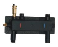
The hydraulic separator CPN MIX-BOX is made of steel. The factory is equipped with insulation sleeve plunger 1/2 "sensor, the automatic air vent 3/8" with check valve 1/2 ", two brass fittings 1" m/f.
